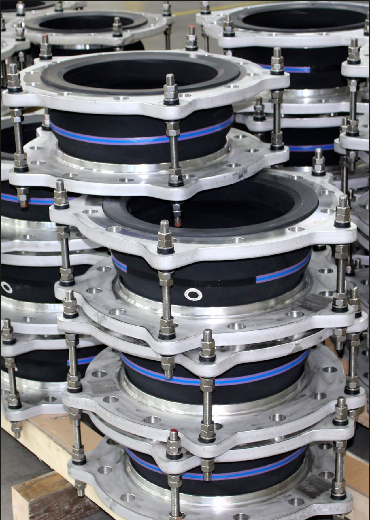
D112M lateral FPM rubber expansion joints of size \varnothing 400 mm with embedded vacuum ring and stainless backing flanges, tie-rods and bearings
