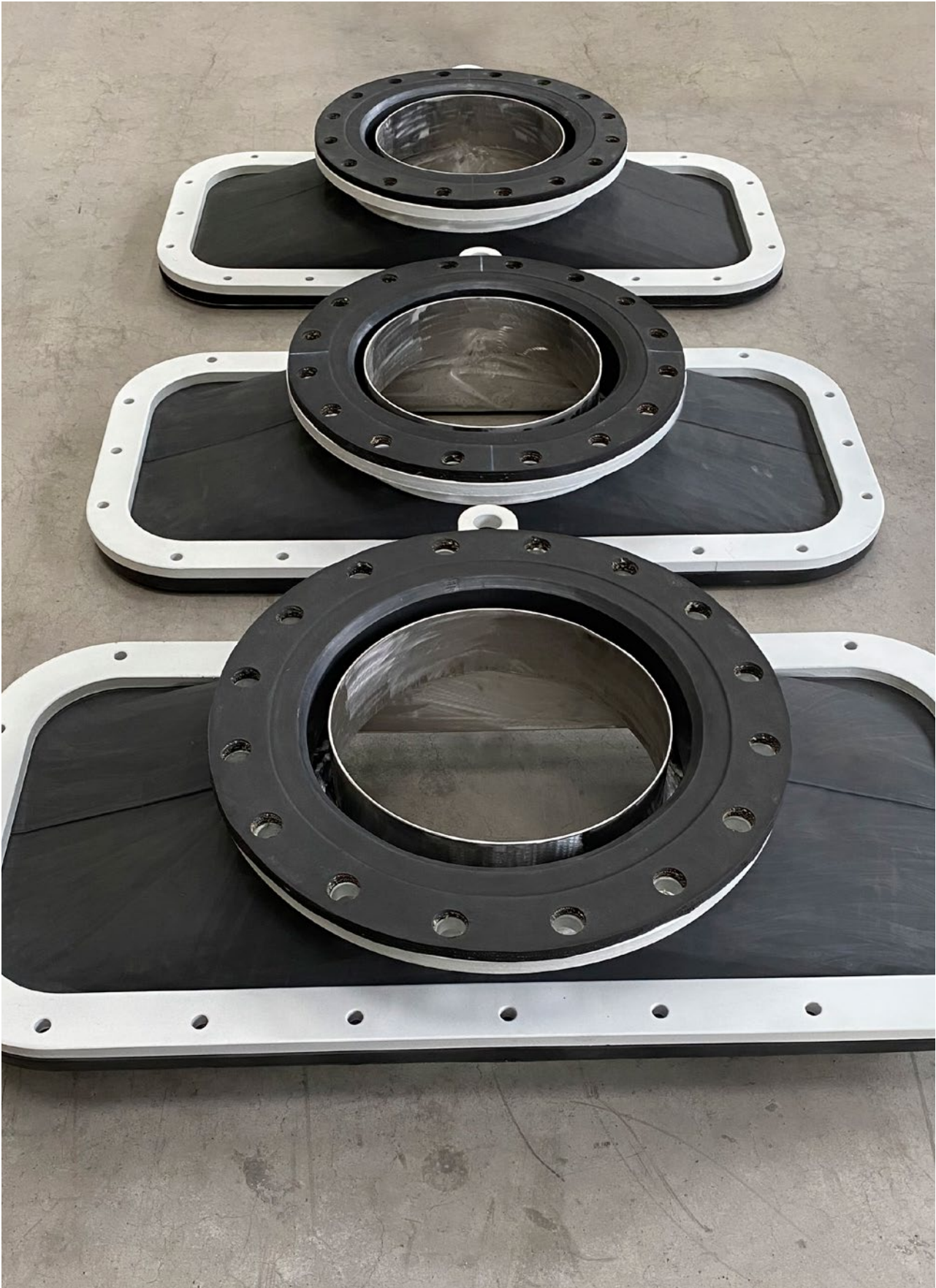
FPM rubber cone from round to rectangular, with stainless steel flow liner test pressure 2,5 bar
