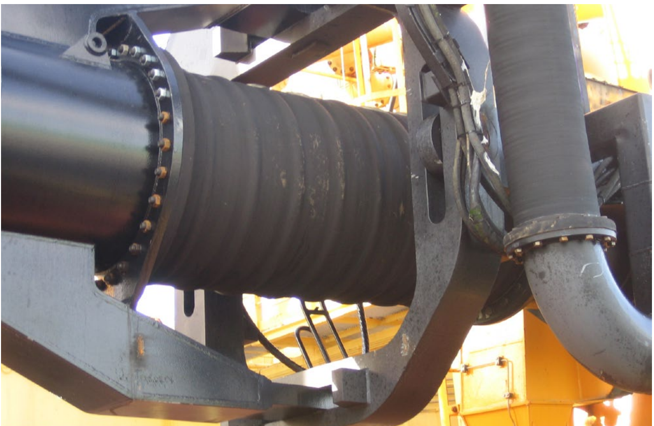
Rubber flanged pipe with embedded steel rings installed on dredger ship
