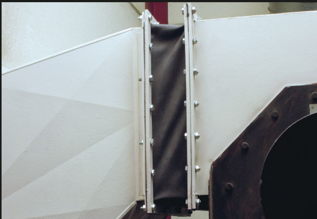
Fabric expansion joint, type EX100 in a solvent extraction facility ∅ 500 x 500 mm, 80 °C
