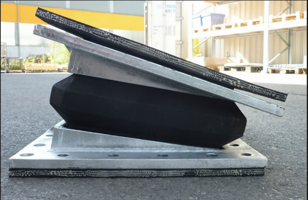
EPDM rubber bellow with angular offset for a coal mill work shop test pressure 15 bar to simulate explosion
