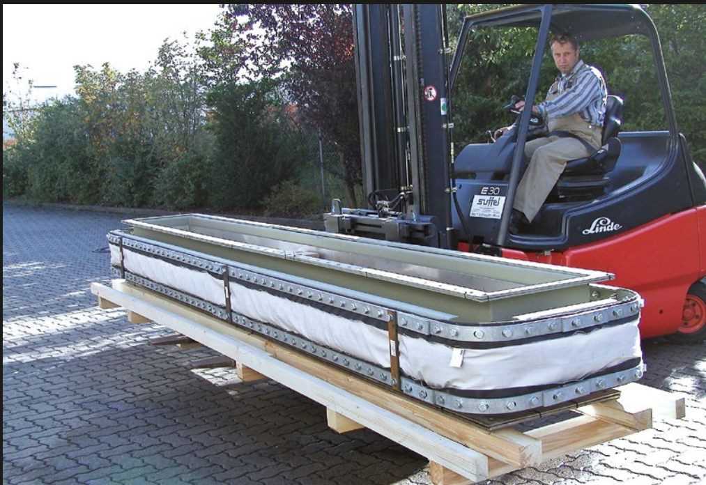
Multilayer expansion joint, type GB300 as a pre-fabricated installation unit for ash discharge in a power plant Ø 5,500 x 600 mm, 750°C
